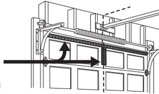
**NOTE:** Many door reinforcement kits provide for direct attachment of the clevis pin and door arm. In this case you will not need the door bracket; proceed to the next step.
