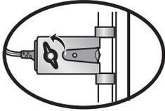
If the receiving sensor is in direct sunlight, switch it with sending sensor so it is on the opposite side of the door.
