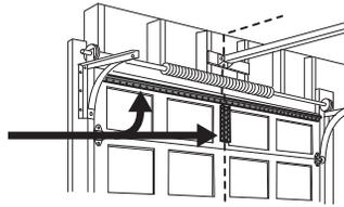
**NOTE:** Many door reinforcement kits provide for direct attachment of the clevis pin and door arm. In this case you will not need the door bracket; proceed to the next step.
